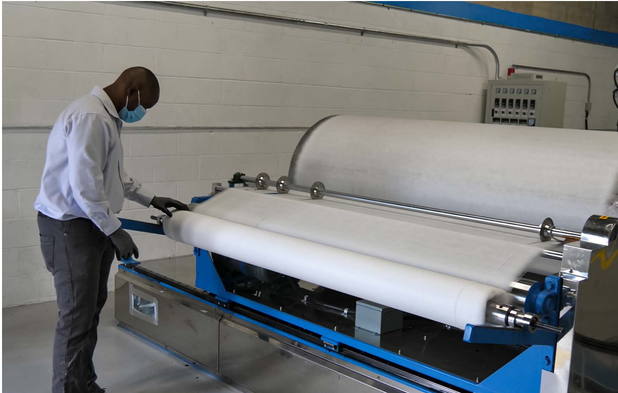
John Rawlins, co-founder of BIG-nano inspecting the Poly (vinyl alcohol) nonwoven fibre mat
